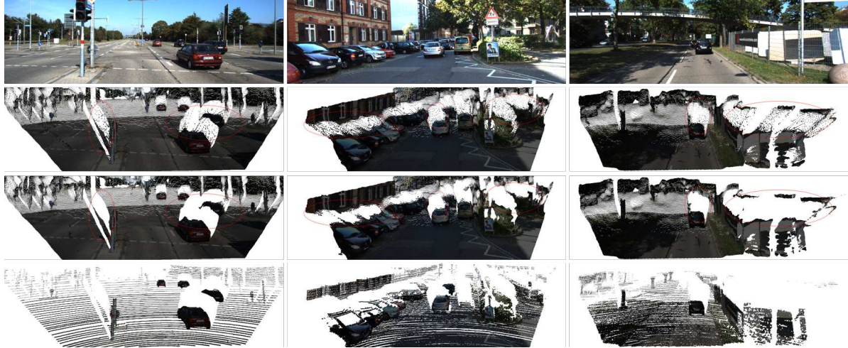
Figure 10. Point cloud converted from disparity with known intrinsic using MeshLab [4]. From top to bottom: the left input image, result from PSMNet [2], result from ours, and groundtruth. Please zoom in for more details.
